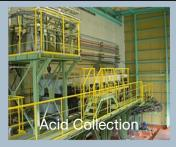
Acid collection machine improves pickling performance by stabilizing acid concentration and iron content while reducing waste from acid treatment to a minimum.
