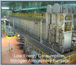
Nitrogen atmosphere furnace reduces impact on the environment by eliminating the need for pickling rods and/or reducing the pickling time after annealing.
